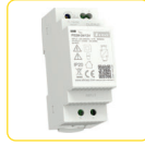
PS2M-24/12V Input: AC 100 - 240 V Output: DC 12 V stab. Load: 2 A/24 W. - short circuit protection - overload protection - overvoltage protection page 44
