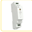
PS1M-15/12V Input: AC 100 - 240 V output: DC 12 V stab. load: 1.25 A/15 W. - short circuit protection - overload protection - overvoltage protection page 44
