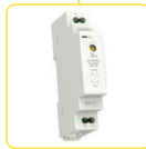
PS1M-15/24V Input: AC 100 - 240 V Input: DC 24 V stab. load: 0.625 A/15 W. - short circuit protection - overload protection - overvoltage protection page 44
