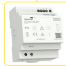
PS4M-92/24V Input: AC 100 - 240 V Input: DC 24 V stab. load: 3.83 A/92 W - short circuit protection - overload protection - overvoltage protection page 44
